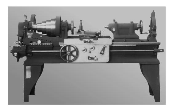
Early cone head engine lathe (c. 1890)
